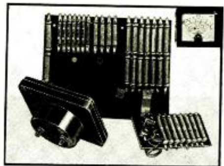
Fig. A. The array of components that go to make up the Tester-Analyzer. The front view of the multi-scale meter (lower-left) is shown in insert.
